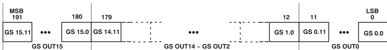
Figure 18. Grayscale Data Packet Format
