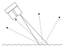
Materials that fall into this category are paper, matte walls, and granite. It is important to note that materials that fit into this category due to observed reflection at visible light wavelengths may exhibit unexpected results in other wavelengths. The near infrared range used by the device may detect them as nearly identical. For example, a black sheet of paper may reflect a nearly identical percentage of the infrared signal back to the receiver as a white sheet.
