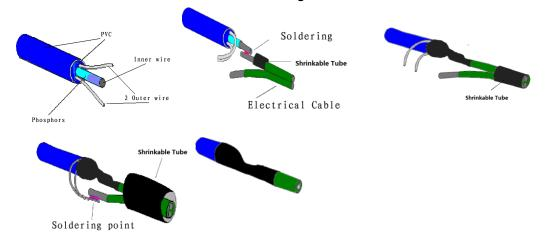
B. Connection between EL Wire and EL Wire
