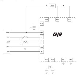
Figure 22-4. Typical bus powered application with 3V I/O.
