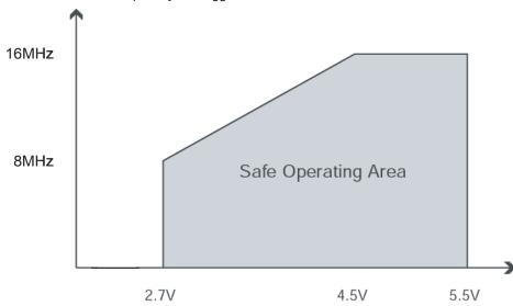
Figure 31-2. Maximum frequency vs. V<sub>CC</sub>, Atmel AT90USB64/128.
