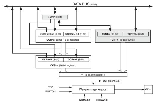
Figure 15-4. Output Compare Unit, block diagram.
