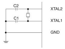
The low power oscillator can operate in three different modes, each optimized for a specific frequency range. The operating mode is selected by the fuses CKSEL3..1 as shown in Table 7-3.
