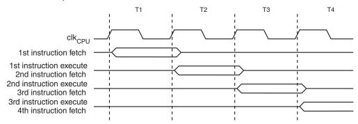
Figure 5-6 shows the internal timing concept for the Register File. In a single clock cycle an ALU operation using two register operands is executed, and the result is stored back to the destination register.
