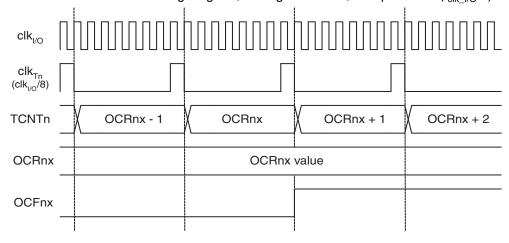
Figure 16-11 on page 156 shows the setting of OCF2A and the clearing of TCNT2 in CTC mode.
