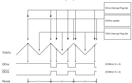
Figure 16-7. Phase correct PWM mode, timing diagram.
