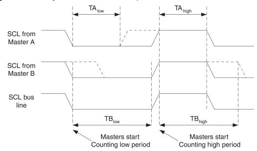
Figure 21-7. SCL synchronization between multiple masters.
