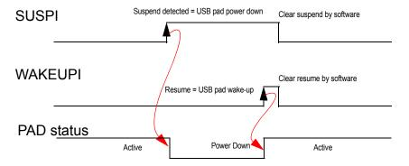
Moreover, the pad can also be put in the "idle" mode if the DETACH bit is set. It come back in the active mode when the DETACH bit is cleared.
