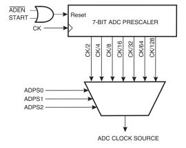
By default, the successive approximation circuitry requires an input clock frequency between 50kHz and 200kHz to get maximum resolution. If a lower resolution than 10 bits is needed, the input clock frequency to the ADC can be higher than 200kHz to get a higher sample rate. Alternatively, setting the ADHSM bit in ADCSRB allows an increased ADC clock frequency at the expense of higher power consumption.
