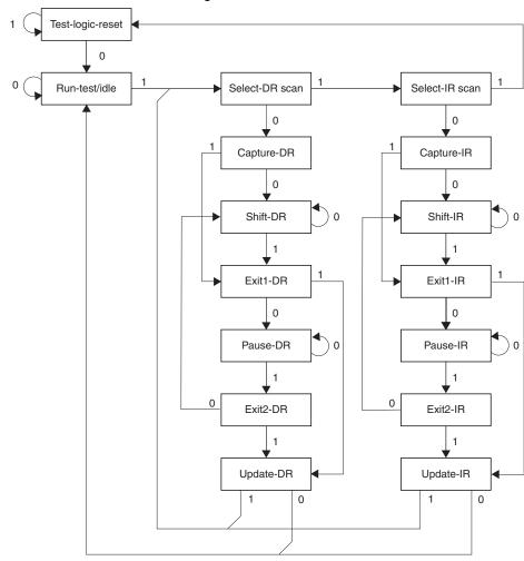
Figure 27-2. TAP controller state diagram.
