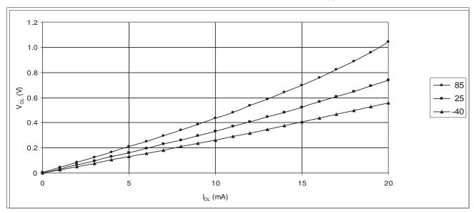
Figure 32-4. Output low voltage vs. output current, all I/Os excluding DP/DM,  $V_{CC} = 5V$ .
