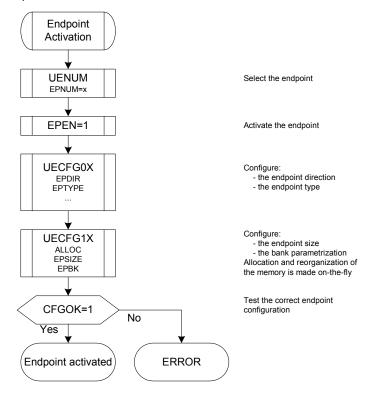
As long as the endpoint is not correctly configured (CFGOK cleared), the hardware does not acknowledge the packets sent by the host.
