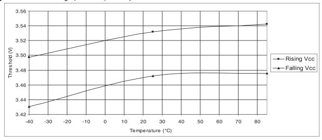
Figure 32-22. BOD voltage (4.3V level) vs. temperature.
