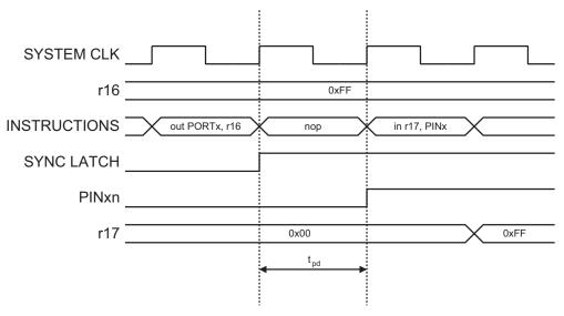
The following code example shows how to set port B pins 0 and 1 high, 2 and 3 low, and define the port pins from 4 to 7 as input with pull-ups assigned to port pins 6 and 7. The resulting pin values are read back again, but as previously discussed, a *nop* instruction is included to be able to read back the value recently assigned to some of the pins.
