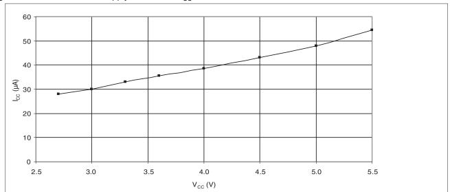
**Figure 32-9.** Power-down supply current vs.  $V_{CC}$ , with BOD enabled, WDT enabled,  $T = 25^{\circ}C$ .
