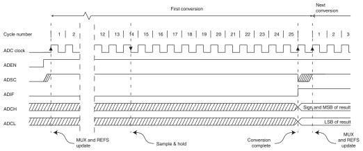
Figure 26-5. ADC timing diagram, single conversion.
