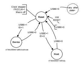
USB Controller state after an hardware reset is 'Reset'. In this state:
