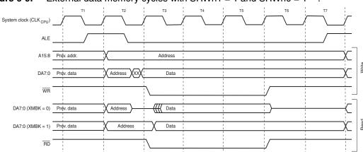
Figure 6-9. External data memory cycles with SRWn1 = 1 and SRWn0 = 1 (1).
