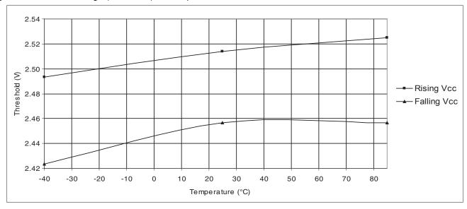
Figure 32-21. BOD voltage (3.4V level) vs. temperature.
