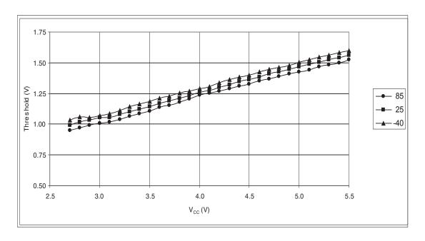
Figure 32-2. Input high voltage vs.  $V_{CC}$ , all I/Os excluding DP/DM, XTAL1 and reset.
