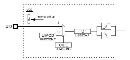
The ID pin can be used to detect the USB mode (Peripheral or Host) or software selected. This allows the UID pin to be used has general purpose I/O even when USB interface is enable. When the UID pin is selected, by default, (no A-plug or B-plug), the macro is in the Peripheral mode (internal pull-up). The IDTI interrupt is triggered when a A-plug (Host) is plugged or unplugged. The interrupt is not triggered when a B-plug (Periph) is plugged or unplugged.
