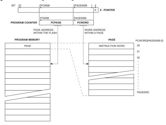
Figure 29-4. Addressing the flash during SPM (1).
