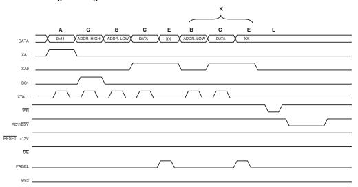
**Figure 30-4.** Programming the EEPROM waveforms.
