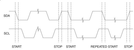
Figure 21-3. START, REPEATED START and STOP conditions.
