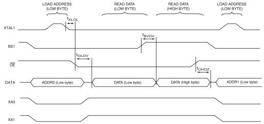
Note: 1. The timing requirements shown in Figure 30-7 (that is,  $t_{DVXH}$ ,  $t_{XHXL}$ , and  $t_{XLDX}$ ) also apply to reading operation.
