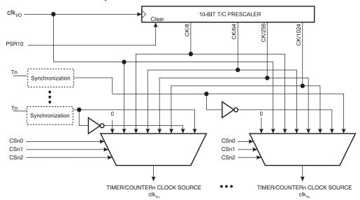
Figure 13-2. Prescaler for synchronous Timer/Counters
