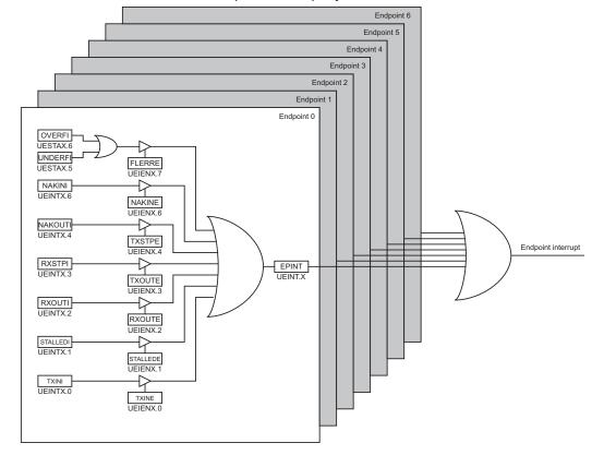
Figure 23-9. USB device controller endpoint interrupt system.
