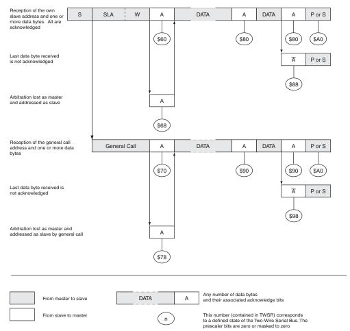
Figure 21-17. Formats and states in the Slave Receiver mode.
