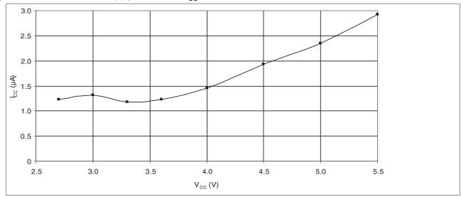
**Figure 32-8.** Power-down supply current vs.  $V_{CC}$ , with BOD disabled, WDT enabled, T = 25°C.
