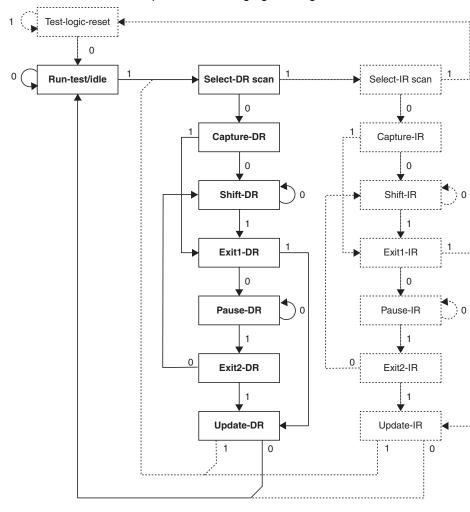
Figure 30-15. State machine sequence for changing/reading the data word.
