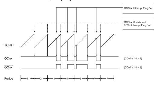
The Timer/Counter Overflow Flag (TOV2) is set each time the counter reaches TOP. If the interrupt is enabled, the interrupt handler routine can be used for updating the compare value.
