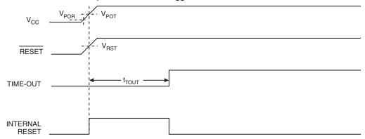
Figure 9-3. MCU start-up, RESET extended externally.
