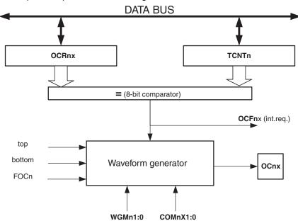
The OCR2x Register is double buffered when using any of the Pulse Width Modulation (PWM) modes. For the Normal and Clear Timer on Compare (CTC) modes of operation, the double buffering is disabled. The double buffering synchronizes the update of the OCR2x Compare Register to either top or bottom of the counting sequence. The synchronization prevents the occurrence of odd-length, non-symmetrical PWM pulses, thereby making the output glitch-free.
