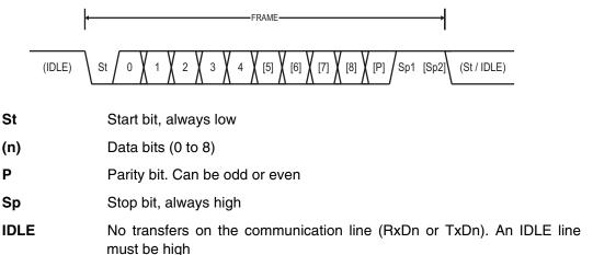
The frame format used by the USART is set by the UCSZn2:0, UPMn1:0 and USBSn bits in UCSRnB and UCSRnC. The Receiver and Transmitter use the same setting. Note that changing the setting of any of these bits will corrupt all ongoing communication for both the Receiver and Transmitter.
