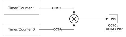
When the modulator is enabled, the two output compare channels are modulated together as shown in the block diagram (Figure 17-1).
