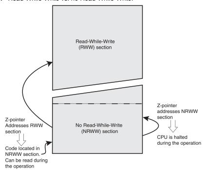
Figure 29-1. Read-While-Write vs. no Read-While-Write.
