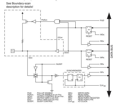
Figure 28-4. General port pin schematic diagram.
