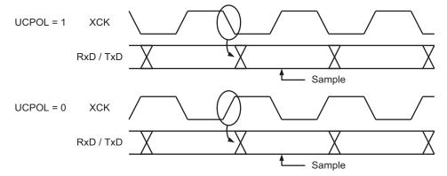
The UCPOLn bit UCRSC selects which XCKn clock edge is used for data sampling and which is used for data change. As Figure 19-3 shows, when UCPOLn is zero the data will be changed at rising XCKn edge and sampled at falling XCKn edge. If UCPOLn is set, the data will be changed at falling XCKn edge and sampled at rising XCKn edge.
