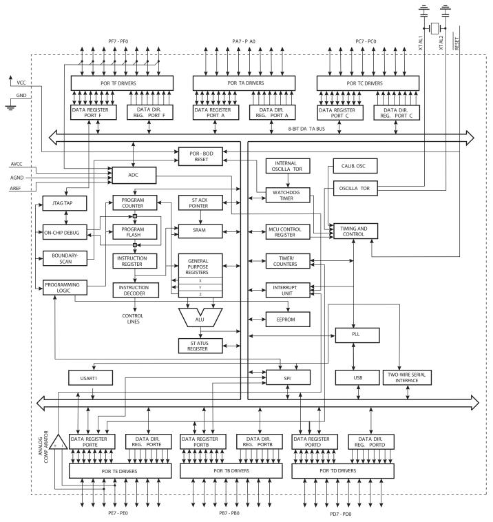
The AVR core combines a rich instruction set with 32 general purpose working registers. All the 32 registers are directly connected to the Arithmetic Logic Unit (ALU), allowing two independent registers to be accessed in one single instruction executed in one clock cycle. The resulting
