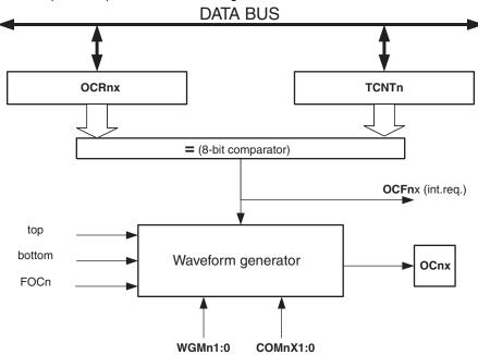
Figure 14-3. Output Compare Unit, block diagram.
