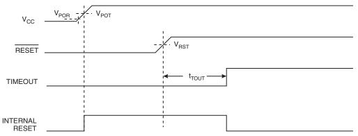
Note: If V<sub>POR</sub> or V<sub>CCRR</sub> parameter range can not be followed, an external reset is required.
