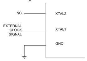
When this clock source is selected, start-up times are determined by the SUT fuses as shown in Table 7-9.
