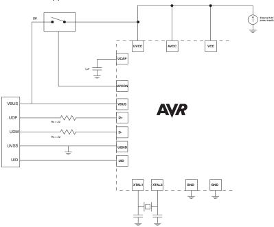
Figure 22-8. Host/OTG application with 5V I/O.
