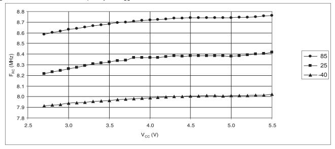
Figure 32-26. RC oscillator frequency vs. temperature.
