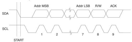
Figure 21-4. Address packet format.
