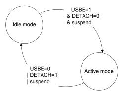
The SUSPI flag indicated that a suspend state has been detected on the USB bus. This flag automatically put the USB pad in Idle. The detection of a non-idle event sets the WAKEUPI flag and wakes-up the USB pad.
