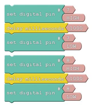
Instead of introducing a new block, we'll be adjusting the value of *Set Digital Pin*'s top pink *Pin Number* block. This value specifies which of the Sandbox's pins we'll be toggling.
