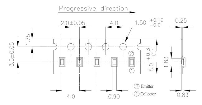
Unit: mm Tolerance: ±0.1mm
