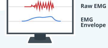
The greater the number of motor units, the more the electrical activity of your muscle increases. The MyoWare will analyze this electrical activity and output an analog signal that represents how hard the muscle is being flexed. The harder you flex, the higher the MyoWare output voltage will go.
