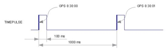
Figure 27: Time pulse signal with the example parameters
