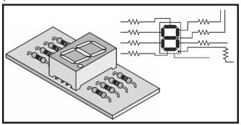
The "8" LED display is mounted on a board and to prevent burning out the display with excess current, permanent resistors have been wired in.
