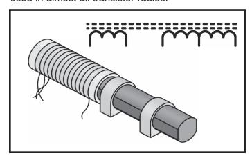
**Transformer:** Did you know that if you were to wrap two wires from different circuits around different ends of an iron bar, and if you were to add current in the first circuit, it will magnetically create current in the second circuit? That's exactly what a transformer is! Transformers are used to isolate parts of a circuit, to keep them from interfering with each other.
