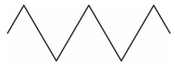
The shape of this wave results from the slow charging of the  $0.1\mu F$  capacitor through the control and the  $100k\Omega$  resistor, and the capacitor's discharge through the PNP and NPN transistors.
