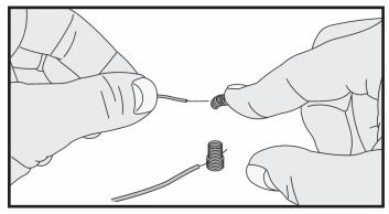
When you have to join to two or three wires into a single spring terminal, be sure that the first wire does not come loose when you attach the second and third wires. The simplest way to do this is to place the spring onto the opposing side where you have connected the first wire.
