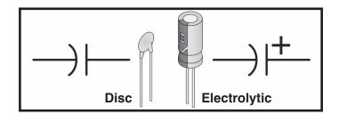
*Disc* - Unlike the electrolytic above, these capacitors have no polarity and can be connected in either way.
