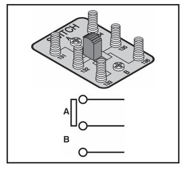
**Key:** The key is a simple switch—you press it and electricity is allowed to flow through the circuit. When you release it, the circuit is not complete because a break is caused in the circuit's path. The key will be used in most circuits often times in signaling circuits (you can send Morse code this way as well as other things).
