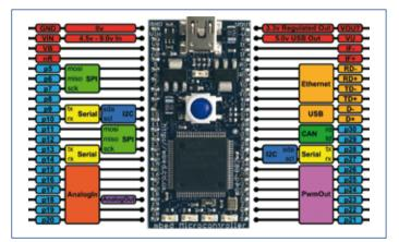
Pinout diagram of mbed NXP LPC1768 board
