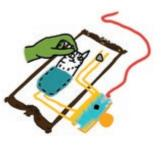
We can turn off the switch by pulling the cat out of the pocket, or by flipping the cat around so that the copper tape doesn't touch the circuit.
