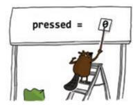
The cool thing about variables is that we can update the stored number. We do this by setting it to another value with the = equal sign. For example, **pressed** = **1** changes **pressed** to equal 1 instead of 0. We use this technique to update our **pressed** variable based on if the button is pressed or not. We program our lights to turn on or off depending on the switch's value. We do this using an **if()** statement. Here is the general structure of the **if()** statement:
