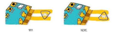
**2. Are any LEDs causing a short circuit?** Make sure that the shiny metal pads of your LEDs are touching only one strip of copper tape. If one pad of an LED is touching two different copper wires, then there is a short circuit and your light will not turn on. In the example below on the right, the wide (+) side is accidentally touching both GND and +3V, causing a short circuit!
