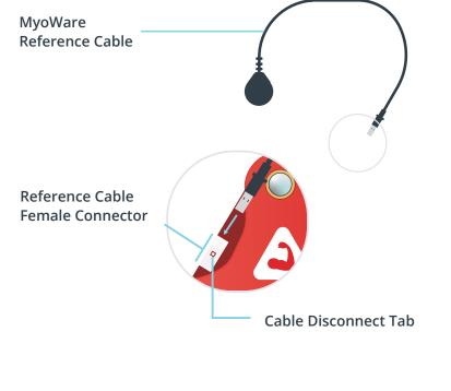
Insert the MyoWare Reference Cable into the female connector located on the left side of the sensor.
