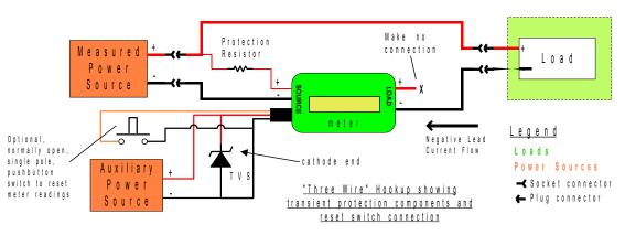
The following diagram shows components added to increase transient voltage protection as well as the use of a pushbutton switch to reset meter readings.
