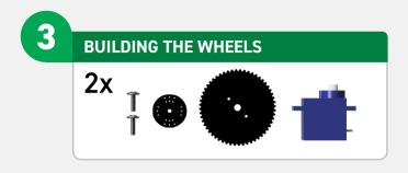
**STEP 1:** Screw the 2 larger screws from the servo packet, through the wheel and into the appropriate holes in the servo attachment. The centre of the horn and the centre of the wheel should be aligned. Press fit the wheel onto the servo and repeat for the opposite side.
