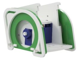
**STEP 7:** Add a wheel (built earlier) and screw the smallest servo screw through the middle to secure it.
