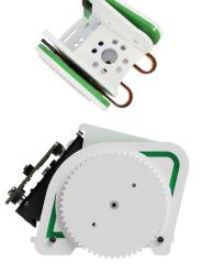
**STEP 3:** Push the SERVO:LITE board fully back inside the :MOVE mini.
