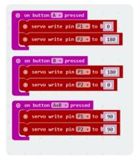
**NOTE:** If the move mini does not travel in a straight line then you can adjust the values to make the servos run at the same speed. You may also need to adjust the trimmer (see pg 17).
