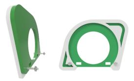
$\ensuremath{\text{STEP}}$  5: Attach to the chassis, slot the nut into the T-joint and tighten the screw.
