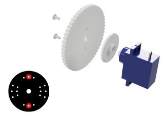
**NOTE:** The screws should go through the holes shown above in red.
