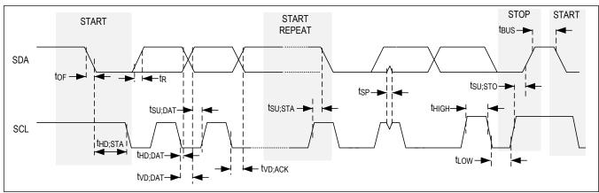
Figure 1. I<sup>2</sup>C Timing Diagram
