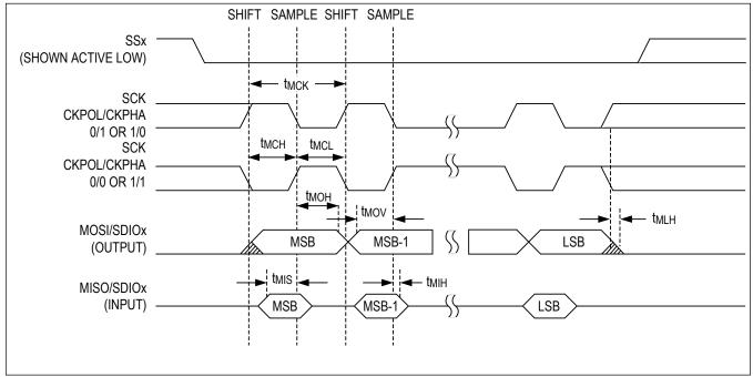
Figure 2. SPI Master Mode Timing Diagram
