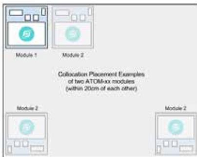
For collocation operation with any other transmitting devices (i.e. - Wifi, Bluetooth, Cellular), it is required that the end product manufacture has the completed product evaluated for compliance with simultaneous transmission requirements. This can be completed by the following:
