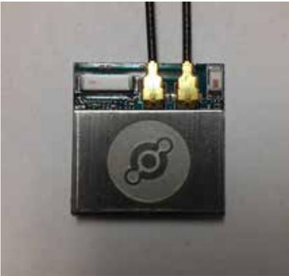
The U.FL to SMA cable that was used during FCC/IC/ETSI testing was a Taoglas CAB.011 cable assembly. This provides a direct SMA connection (for external antennas) to the module via the U.FL connector.
