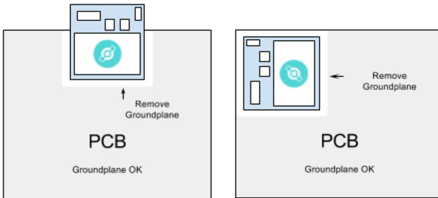
Based on the above recommendations, there may be situations where you cannot place the module near an edge. This may force the module to be buried within the center groundplane of the host base board. Even though this is not recommended due to the dramatic decrease in chip antenna performance, the U.FL connections will still provide adequate RF performance to the external antenna of choice. As long as the ground plane can be minimized under the module as shown in the following figure.
