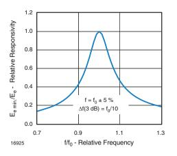
Fig. 5 - Frequency Dependence of Responsivity
