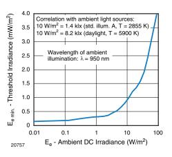
Fig. 6 - Sensitivity in Bright Ambient
