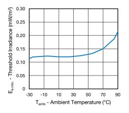
Fig. 9 - Sensitivity vs. Ambient Temperature
