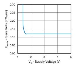
Fig. 13 - Sensitivity vs. Supply Voltage
