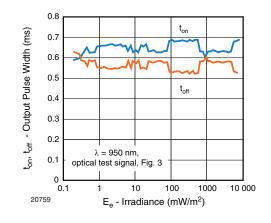
Fig. 4 - Output Pulse Diagram
