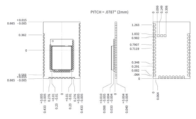
Mechanical drawings XBee 3 micro antennas
