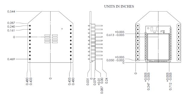
XBee 3 through-hole - U.FL antenna
