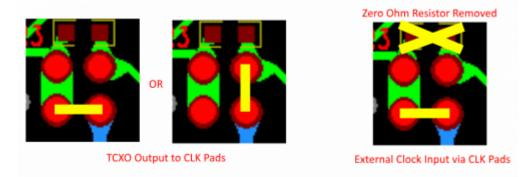
An example of CLK daisy chaining is shown below. One dongles TCXO is connected to two other dongles who have disconnected clocks.
