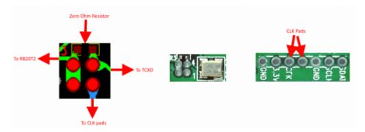
The first position allows you to output the dongles clock to the CLK pads. The second position allows you to input an external clock.
