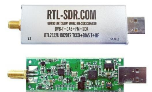
The RTL-SDR Blog V3 is an improved RTL-SDR dongle. RTL-SDR dongles were originally designed for DVB-T HDTV reception, but they were found by hardware hackers to be useful as a general purpose SDR. The standard dongles are okay for DVB-T reception, but are just barely suitable for SDR users/experimenters. The RTL-SDR Blog V3 was redesigned with SDR user needs in mind, instead of DVB-T HDTV users who typically have more relaxed requirements.
