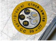
The CelsiClock® multi-level label combines five levels on a minimal area. This CelsiClock® was on a part going through thermal treatment. Levels 99, 121 and 143 °C have blackened. QC of parts manufacturing now has proof of sufficient treatment level, part can be released.
