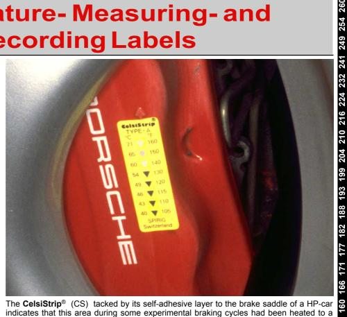
The **CelsiStrip**<sup>®</sup> (CS) tacked by its self-adhesive layer to the brake saddle of a HP-car indicates that this area during some experimental braking cycles had been heated to a maximal level of 54°C. The still original white temperature levels had not been reached. Only the Celsi® temperature sensing technique allows such a quick, easy to apply, really low cost temperature measuring and recording set-up.
