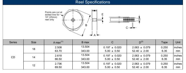
Dimension "E": This is a non-critical dimension that does not have a tolerance in the standard.
