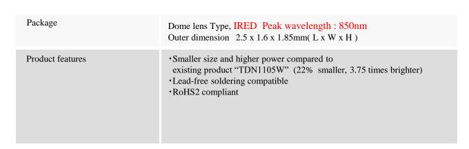
This product is classified "Exempt" according to "Photobiological safety of lamps and lamp systems: IEC62471". (Calculated at radiant intensity 50 mW/sr)
