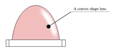
Please adjust the load, the pick up point, the nozzle diameter and etc. before mounting because the over load can cause the breakage of the surrounding of LED.
