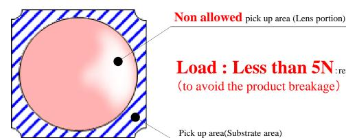
Load : Less than 5N reference (to avoid the product breakage)
