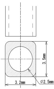
Nozzle with chamfering is recommended
