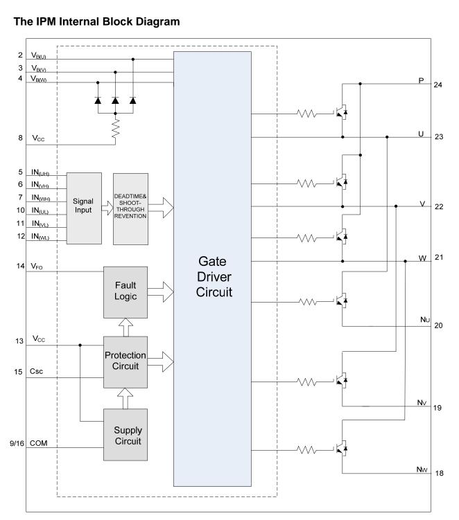
Figure 3. IPM Internal Block Diagram
