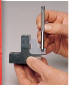
Left: S167CHZ Radius Gauge Set with 25 gauges and holder in case Above: Gauging radii using gauge with holder
