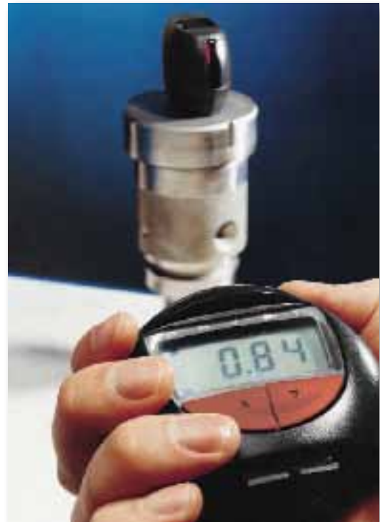
The SR100 uses an infra-red (IrDA) link between the upper and lower units to provide remote, cable free operation up to a distance of one metre (40").
