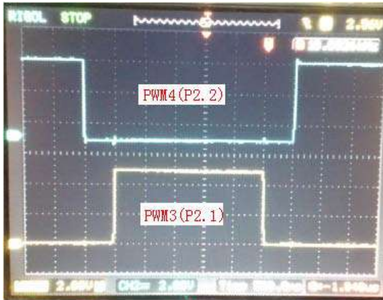
图3: 某个时刻PWM波形, 2V/DIV, 500nS/DIV
