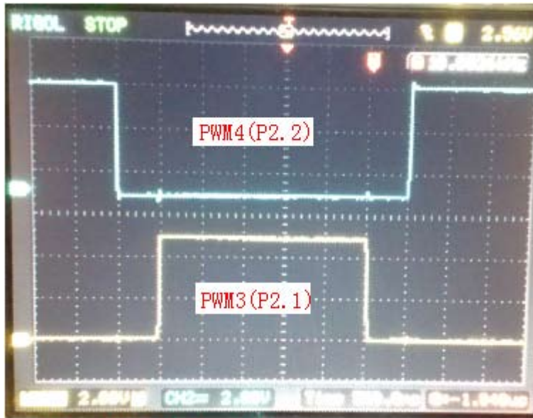
图3: 某个时刻PWM波形, 2V/DIV, 500nS/DIV
