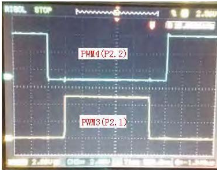
图3: 某个时刻PWM波形, 2V/DIV, 500nS/DIV
