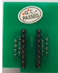
Transition Socket of SOP16 or SOP8(back)
