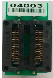
Transition Socket of SOP28 or SOP20(front)
