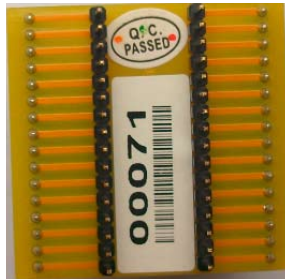
Transition Socket of SOP32(back)
