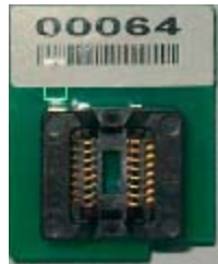
Transition Socket of SOP16 or SOP8(front)
