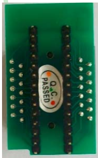
Transition Socket of SOP28 or SOP20(back)
