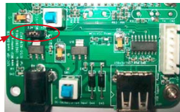
单片机电源电压的选择跳线短接MCU-VCC和5V电源管脚
