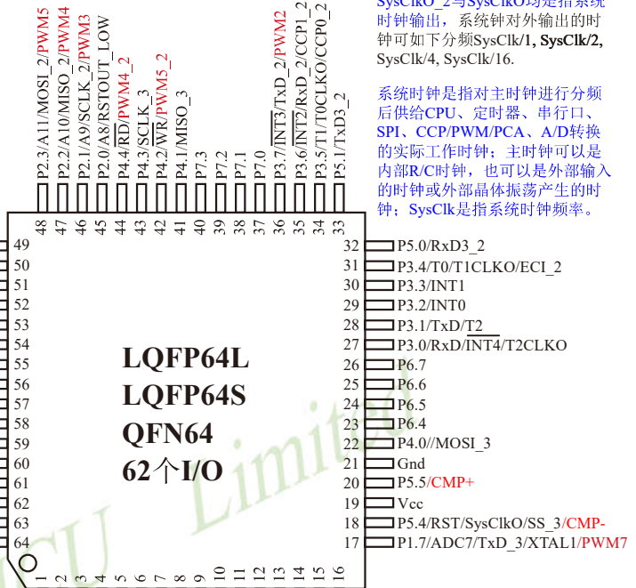
LQFP64L (16mm x 16mm) LQFP64S (12mm x 12mm) QFN64 (9mm x 9mm)
