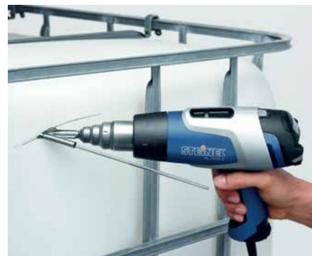
Repairing. Welding PVC water tank.
