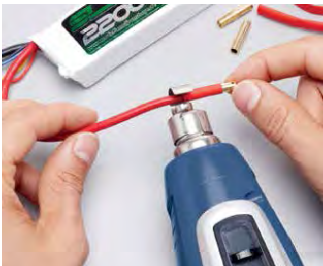
Heat-shrinking. Secure standing for hands-free work.
