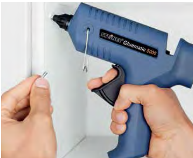
Securing. Fixing shelf supports in cabinets.
