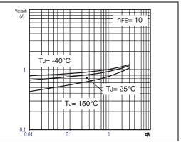
Figure 6. Collector-emitter saturation voltage
