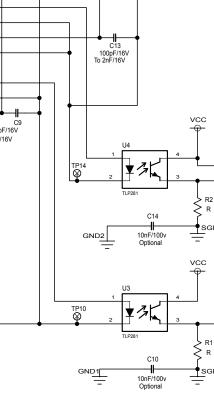
Figure 6. STEVAL-IFP035V1 schematic - isolated digital input /TP1 JP5 ∏ JP6 GND2 TP13
