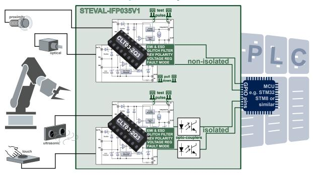
Figure 2. Block diagram
