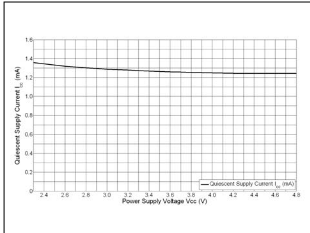
Figure 2. Current consumption vs. power supply voltage
