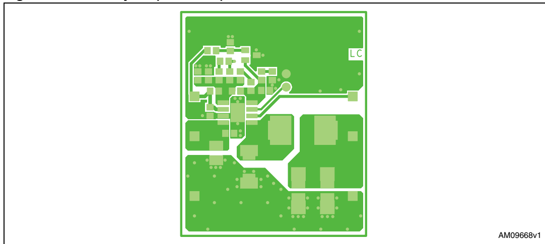
Figure 25. PCB layout (front side)
