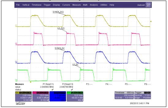
Figure 44. Two regulators synchronized
