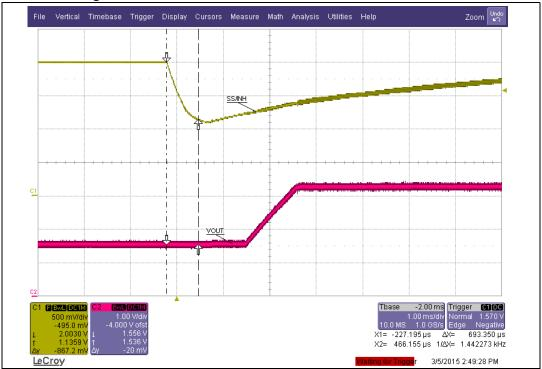
Figure 9. External soft-start after UVLO or thermal shutdown
