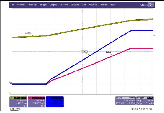
Figure 11. Ratiometric startup operation
