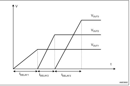
Figure 12. Output voltage sequencing
