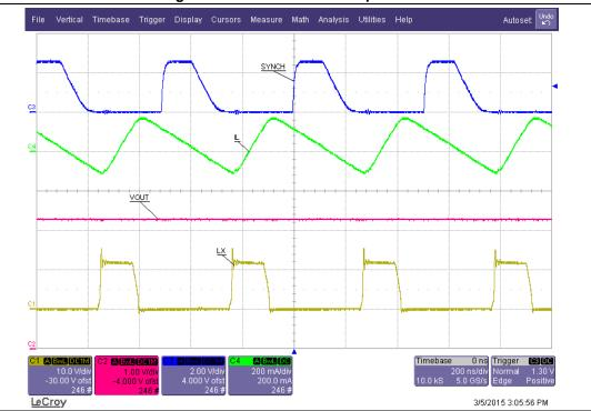
Figure 16. Low noise mode operation
