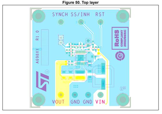
The layout of the board is shown in *Figure 50* and in *Figure 51*.
