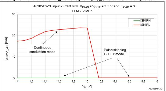
Figure 27. Current from V<sub>IN</sub> while regulating V<sub>OUT</sub> = 3.3 V at zero output load
