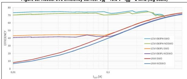
Figure 59. A6985F3V3 efficiency curves:  $V_{IN}$  = 13.5 V - f<sub>sw</sub> = 2 MHz (log scale)
