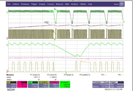
Figure 34. Overvoltage operation
