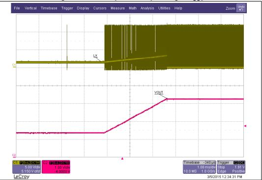
Figure 6. Soft-start phase with precharged COUT
