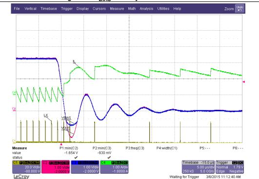
Figure 33.  $V_{BIAS}$  in heavy short-circuit event
