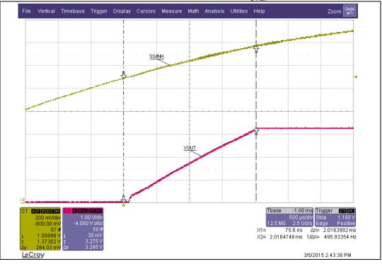
Figure 8. External soft-start network V<sub>STEP</sub> driven
