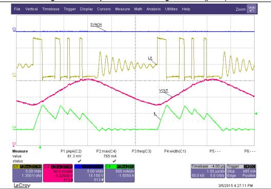
Figure 23. LCM operation over loading condition (part 2)
