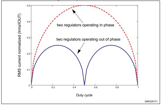
Figure 43 shows two regulators not synchronized.
