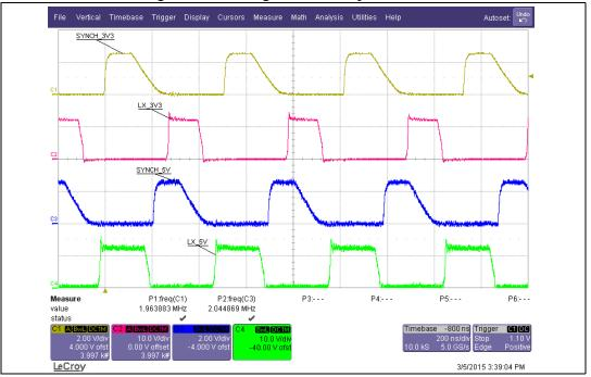
Figure 43. Two regulators not synchronized
