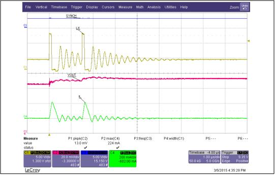
The LCM operation satisfies the requirements of the unswitched car body applications (KL30). These applications are directly connected to the battery and are operating when the engine is disabled. The typical load when the car is parked is represented by a CAN transceiver and a microcontroller in sleep mode (total load is around 20 - 30  $\mu$ A). As soon as the transceiver recognizes a valid word in the bus, it awakes the  $\mu$ C and the rest of the application.
