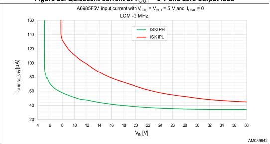
Figure 26. Quiescent current at V<sub>OUT</sub> = 5 V and zero output load
