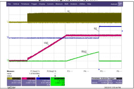
Figure 41. Voltage supervisor operation
