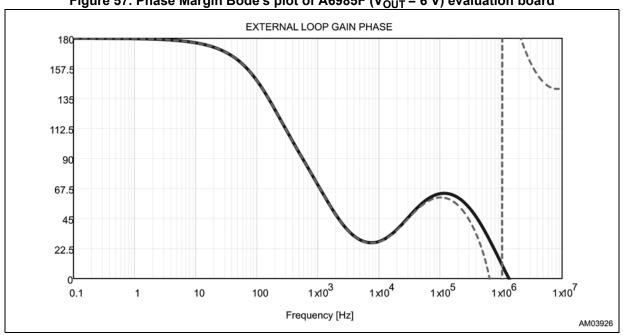
Figure 57. Phase Margin Bode's plot of A6985F (V<sub>OUT</sub> = 6 V) evaluation board
