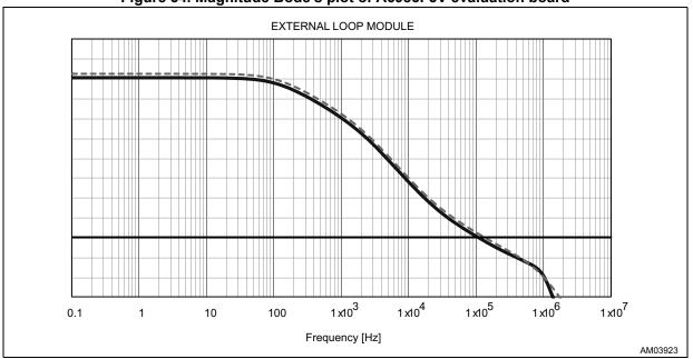
Figure 54. Magnitude Bode's plot of A6985F5V evaluation board
