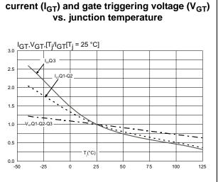
Figure 9. Relative variation of gate triggering
