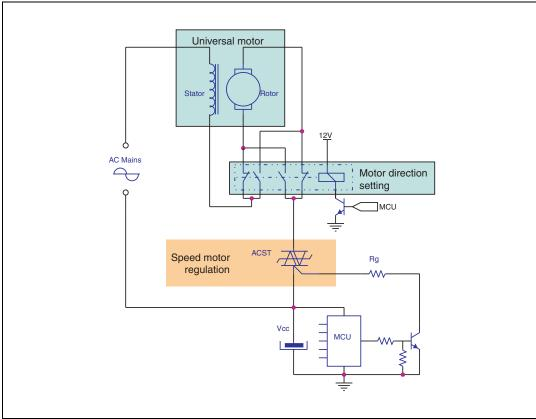
Figure 16. Universal drum motor control – typical diagram
