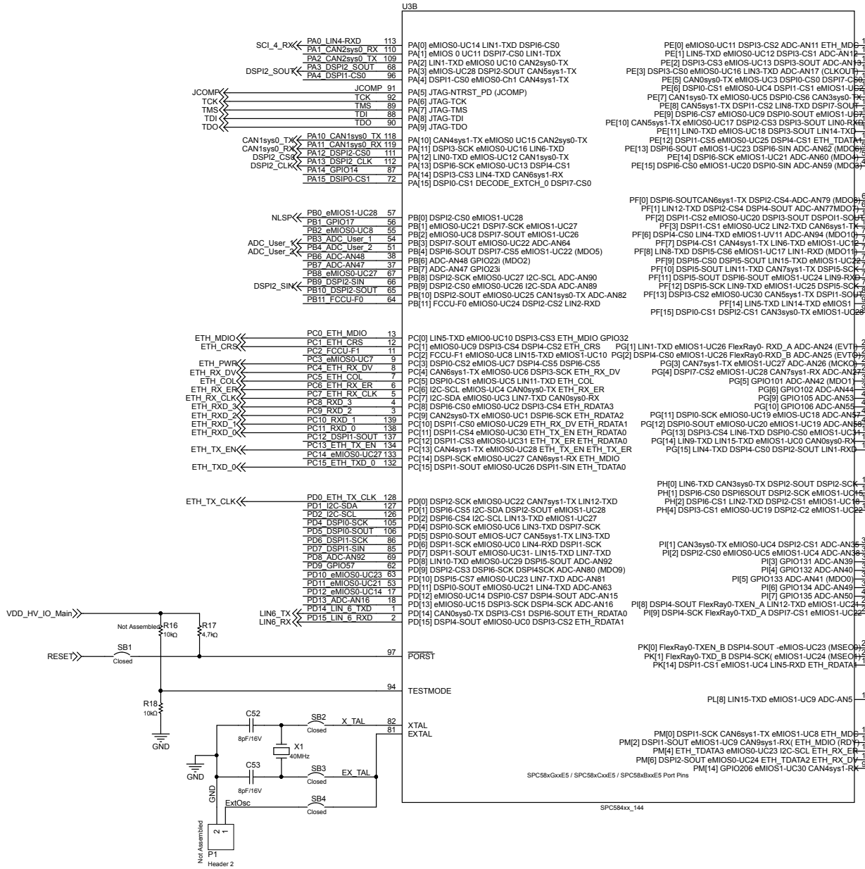
Figure 12. AEK-MCU-C4MLIT1 schematic - MCU I/O signals
