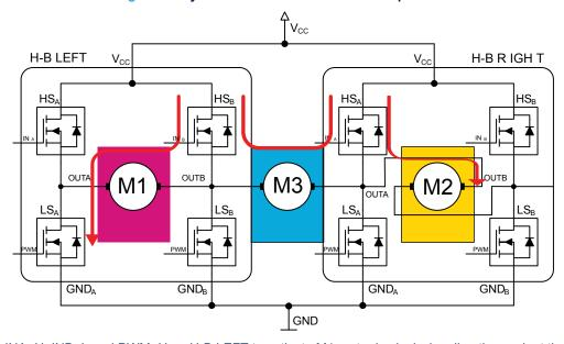
Step 2. Set INA=H, INB=L and PWM=H on H-B LEFT to activate M1 motor in clockwise direction and, at the same time, set INA=L, INB=H and PWM=H on H-B RIGHT to activate M2 motor in clockwise direction. M3 motor is braked to GND.
