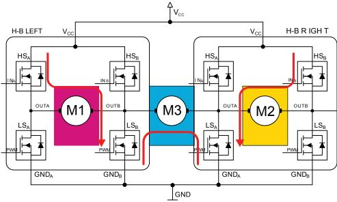
Step 2. Set INA=L, INB=H and PWM=H on H-B LEFT to activate M1 motor in counterclockwise direction and, at the same time, set INA=H, INB=L and PWM=H on H-B RIGHT to activate M2 motor in clockwise direction.
