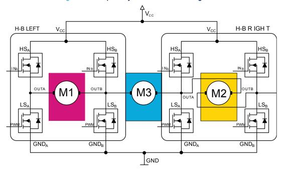
Figure 10. Example of synchronized motor configuration
