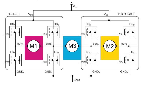
Figure 3. Multi-motor configuration for three motors
