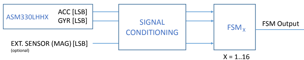
Figure 2. State machine in the ASM330LHHX
