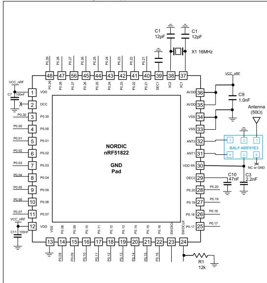
Figure 8. Application schematic
