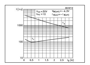
Figure 10. Resistive load switching time
