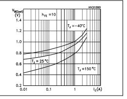
Figure 8. Base-emitter on voltage
