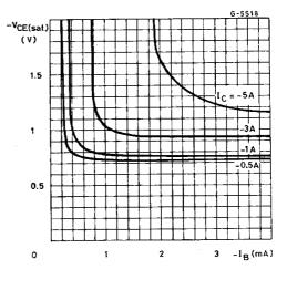
Saturated Switching Characteristics (NPN types)
