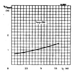
Collector Emitter Saturation Voltage (NPN types)
