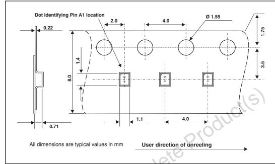
Figure 10. Flip Chip tape and reel specifications
